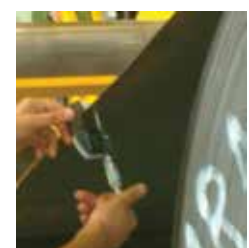
• Digital micrometer for material thickness check
