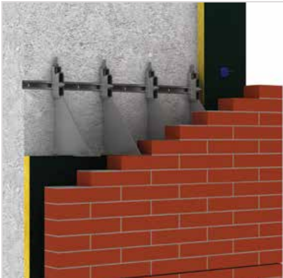
• Perspective picture of brick facing installation with FIX-U brackets.
