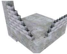
Block work wall
