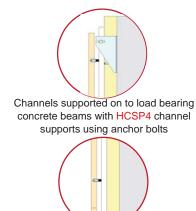
Stone installation is made with BA Body Anchors on to channels with self tabbing screws
