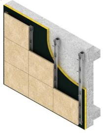
Sub Channel Fixing System with Vertically & Horizontally spanned channels
