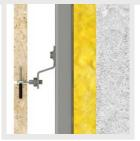
Dead Load Capacity: 400 N Wind Load Capacity: 316 N
