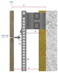
K: projection size Fdw: dead Load Ws: wind pressure C: wall cavity I: insulation thickness CH: channel height F: anchor forming size
