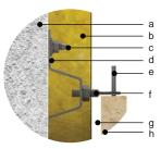
When designing fixing systems by using pin system, atachments to stone can be made at either horizontal or vertical joints. this is determined according to the pattern of the stone layout. Adjustable anchors are used and can be fixed directly to load bearing walls or fixed on channel systems.
