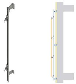
HMPA-HC2 Sub Channel Fixing System
