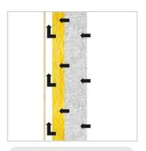
The air gap prevents heat accumulation and damage due to moisture. Load-bearing outside walls and the insulation in particular remain dry and in proper function. The overall construction continues to allow diffusion of moisture.
