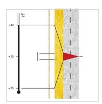
The suspended rear ventilated facade shields the building from strong thermal loading
